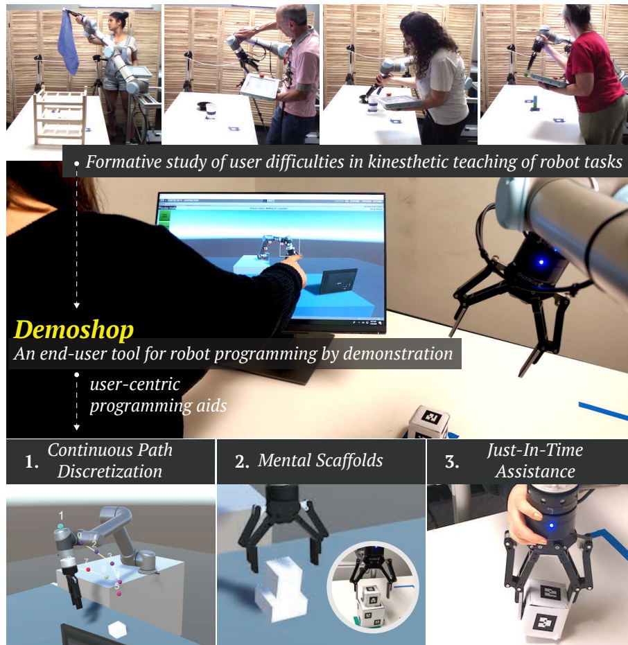
Figure 1: Based on user difficulties and needs that we observed in a formative study where users used kinesthetic teaching to program a robot, we developed Demoshop, an end-user robot programming tool that augments user capabilities in specifying motion demonstrations. Demoshop provides user-centric programming aids in the form of continuous path discretization, mental scaffolds, and just-in-time assistance.
